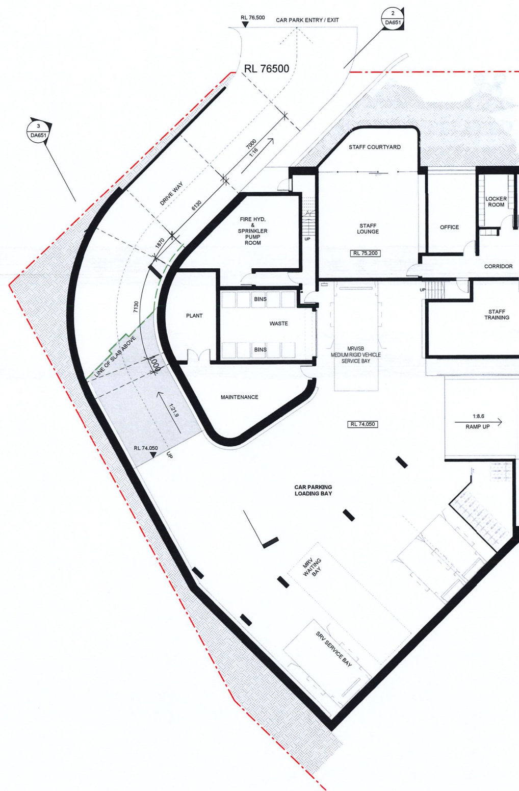
1 DRIVEWAY RAMP PLAN - BASEMENT DA651 1 : 150
